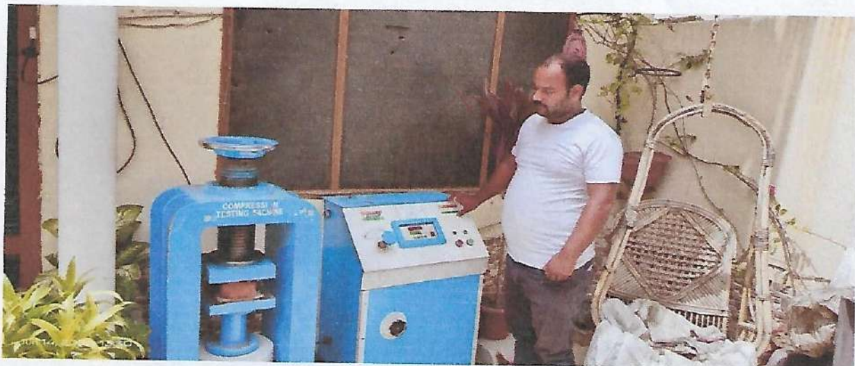
COMPRESSIVE TESTING MACHINE DURING BRICK TEST
