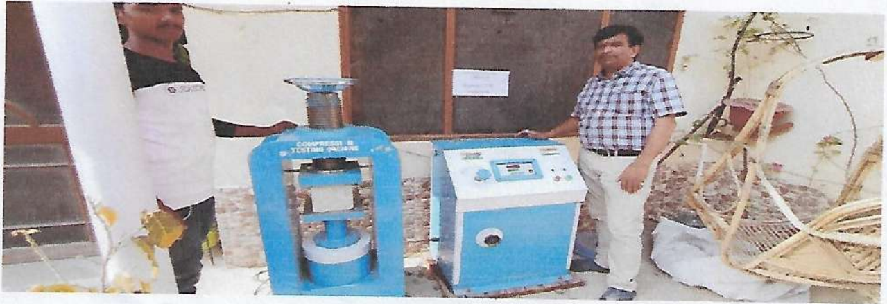
CUBE COMPRESSIVE TESTING MACHINE FOR BRICK, CONCRETE CUBE ,C.C.PAVER
